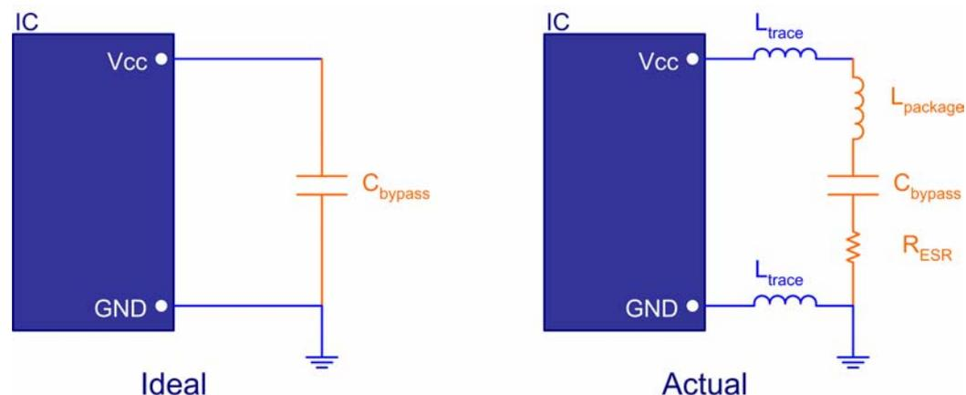
**Figure 9: Realistic De-coupling**
