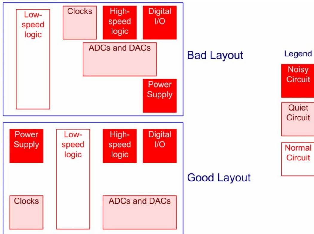
**Figure 1: Isolation of Functional Blocks on a PCB**
