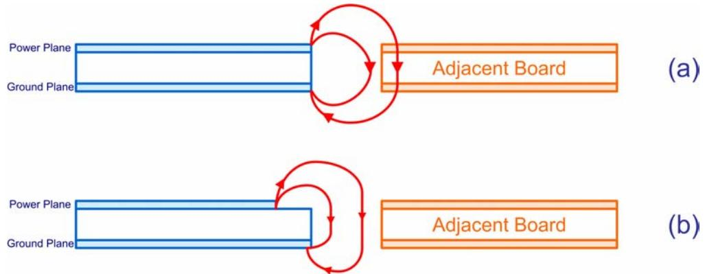
**Figure 5: Edge Emissions from Power and Ground Planes**
