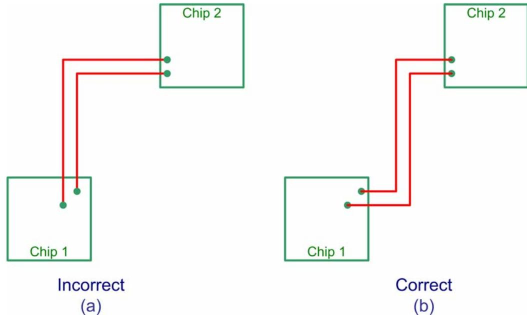
**Figure 7: Routing a Differential Pair Around a Bend**
