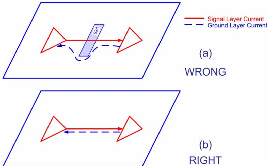
**Figure 4: A Slot in a Ground Plane**
