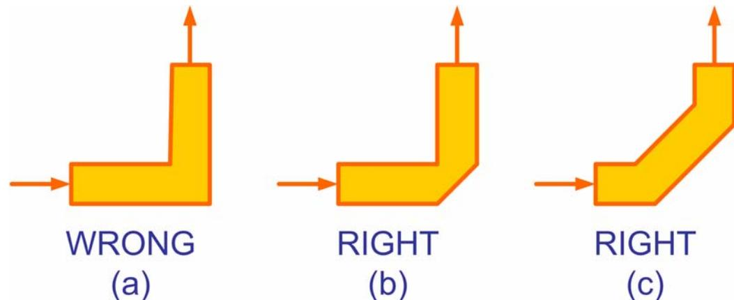
**Figure 6: High-Speed Corners**
